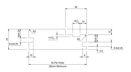
Extension Head Length = Lining Head Length Extension Head Rebate Length = Extension Head Length - 50mm Extension Head Rebate Depth = 9mm Extension Jamb Length = Lining Jamb Length + 15mm
